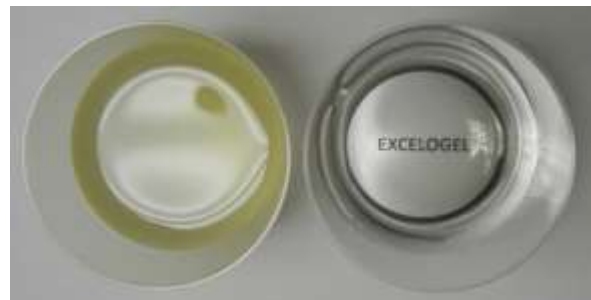
Broken guar (left) and EXCELOGEL (right) to show much cleaner breakdown for low formation damage
