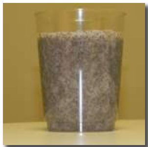
Crosslinked EXCELOGEL to show excellent proppant loading capacity
